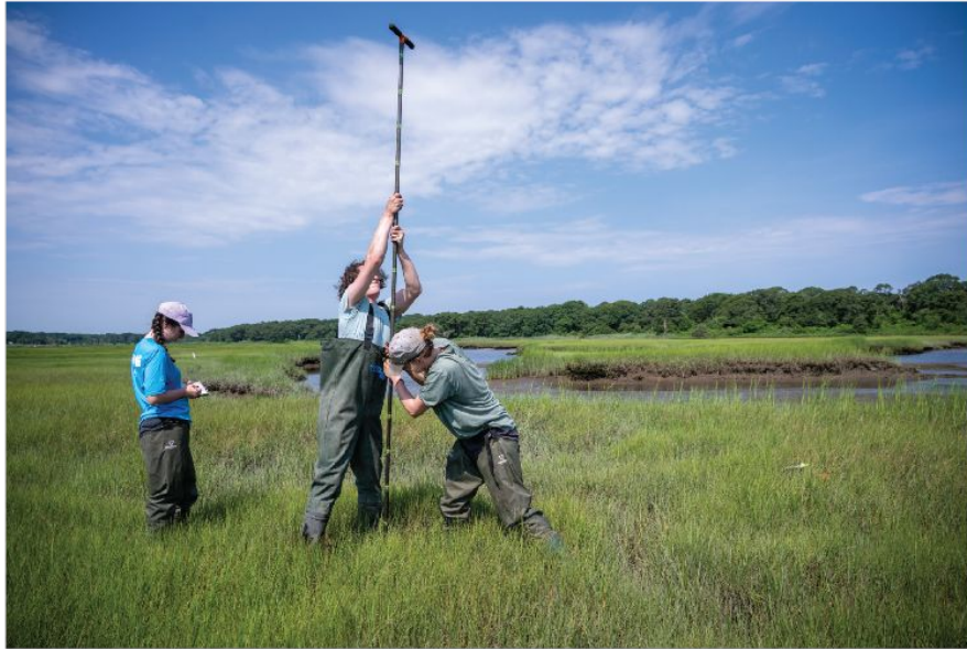
Meg, Dylan, and Sintra measuring peat thickness of a salt marsh on Cape Cod, MA
