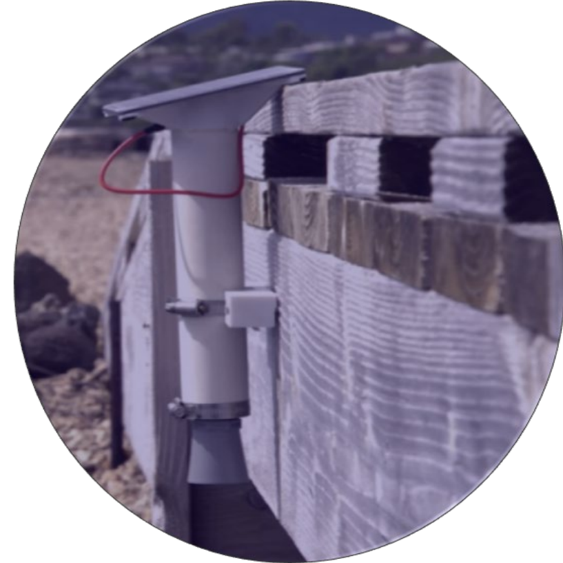
Ultrasonic flood sensor (Photo courtesy of Hohunu)
